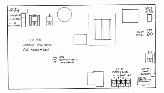
Step Five Verify the threshold adjustment works correctly by increasing the speed of the running belt.
