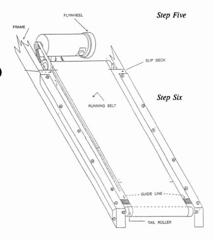
Remove the tailroller bolts by using a T Hex Key. Turn bolts counter-clockwise to remove. Place the tailroller to the side.
